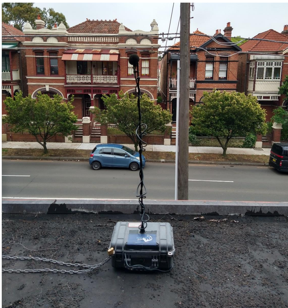
Figure 3: Noise Monitor on Stanmore Road Façade
